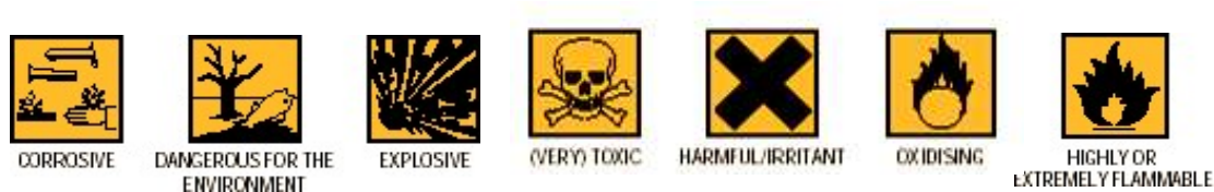
Sample of Hazard Warning Symbols
